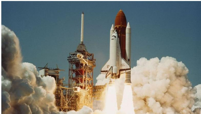
apparatus. Two mammoth white rockets on the side of the shuttle are solid rocket boosters. They produce a total of five million pounds of thrust. After two minutes and 15 seconds, these two rockets are jettisoned and fall harmlessly into the ocean.
